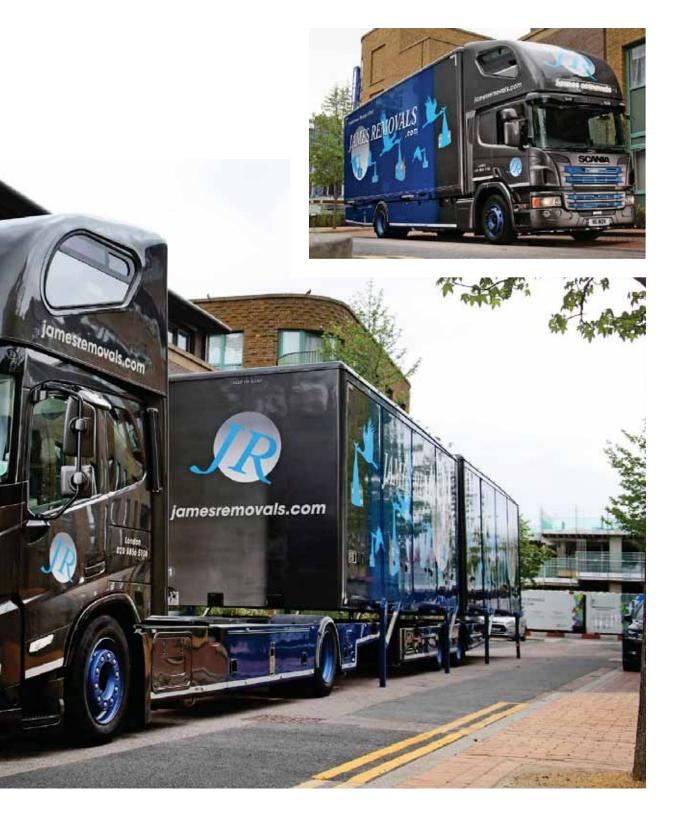
resulted in the trucks being only 20mm higher than our conventional vehicles and the trailer, with its smaller wheels, was a full 250mm lower."
